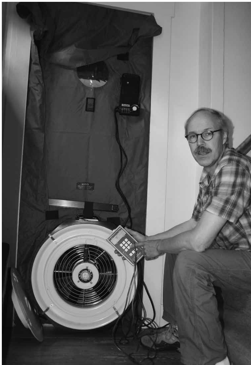
The "blower door test" is a means for measuring air infiltration, and can also be used after weatherization measures have been performed to determine their effectiveness. Above, technician Bruce Courtot, then with VEIC, performs a test at a home in Plainfield in 2010.
