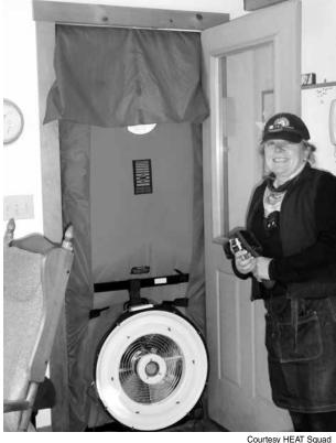
Auditor Sally Ayers with **HEAT Squad performs** a blower door test. The test determines where the home is leaking warm air to the outdoors. This helps HEAT Squad and the homeowner prioritize where and what kind of weatherization to install to reduce air infiltration the most. A reduction of 10 percent or more triggers Efficiency Vermont rebates. To request a home audit, contact HEAT Squad in the Northeast Kingdom; Capstone Community Action in the other counties WEC serves.
